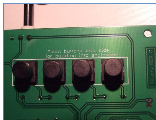
Buttons mounted on solder side (for enclosure use)
