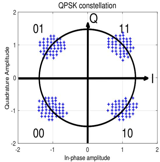
FIG. 4. Constellation diagram for the QPSK test channel carrying a DVB-S protocol in the presence of reflections and an interfering analog wide-band channel with 27 MHz frequency modulation width at the same carrier frequency.
